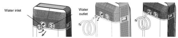
Once the water hose is connected to the air conditioner, there are 5 ways to connect the water hose to the tap. Care must be taken to ensure that the connection is tight. The 3 different hose connectors are designed for different taps.
